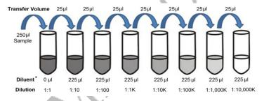
\* Depending upon the sample type being run, it is important to use the same Assay Diluent to dilute the samples, resuspend the Standard Stock, and to prepare the Standard dilution series:
